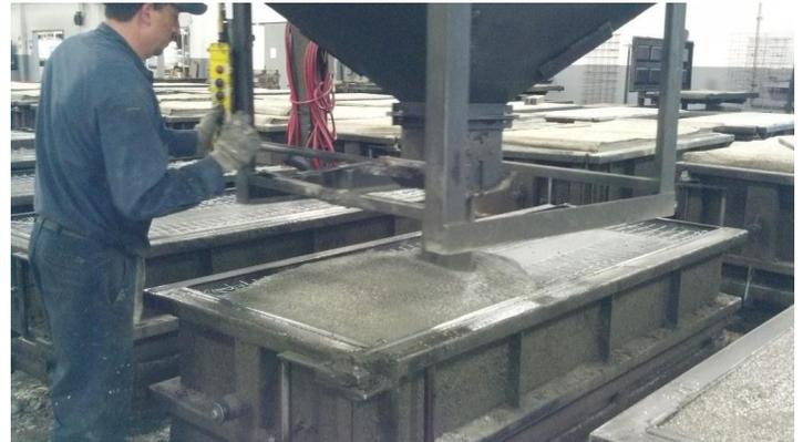
**Worker pours concrete into a mold for these locally-produced vaults.**
